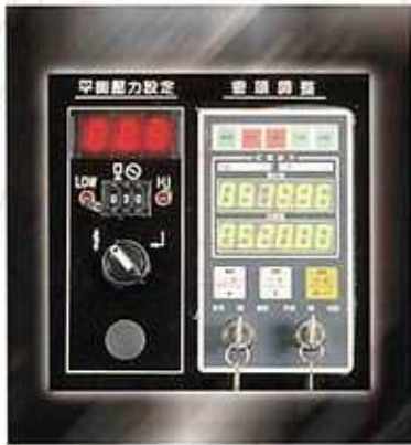
Digital Slide Adjustment Digital slide adjustment readout is recessed in front right side of slide face and indicates the die height in 0.1 mm scale.
